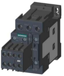
CONTACTOR, AC-3, 11KW/400V, 2NO+2NC, DC 24V, 3-POLE, SZ S0 SCREW TERMINAL REMOVABLE AUX. SWITCH
