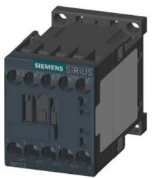
4NO CONTACTOR, AC1: 18A AC 24V 50/60HZ 4-POLE, 4NO, SZ: S00, SCREW TERMINAL
