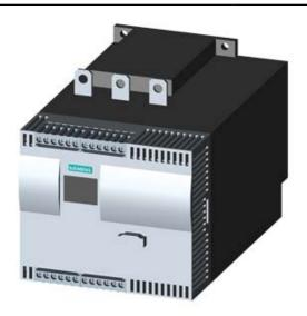
SIRIUS SOFT STARTER, VALUES WITH 575 V, 50 DEG., STANDARD: 100A, 75HP, INSIDE-DELTA CIRCUIT 3: 173A, 150HP, 400-690 V AC, 115 V AC, SCREW TERMINALS
