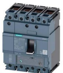
CIRCUIT BREAKER 3VA1 IEC FRAME 160 BREAKING CAPACITY CLASS H ICU=70KA @ 415 V 4-POLE, LINE PROTECTION TM240, ATAM, IN=100A OVERLOAD PROTECTION IR=70A ...100A SHORT CIRCUIT PROTECTION II=5...10 X IN NEUTRAL PROTECTION 50% CABLE CONNECTION
