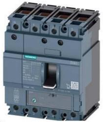
CIRCUIT BREAKER 3VA1 IEC FRAME 160 BREAKING CAPACITY CLASS S ICU=36KA @ 415 V 4-POLE, LINE PROTECTION TM220, ATFM, IN=125A OVERLOAD PROTECTION IR=87,5A ...125A SHORT CIRCUIT PROTECTION II=10 X IN NEUTRAL PROTECTION 50% CABLE CONNECTION
