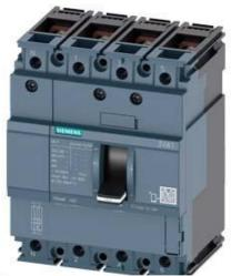
CIRCUIT BREAKER 3VA1 IEC FRAME 160 BREAKING CAPACITY CLASS H ICU=70KA @ 415 V 4-POLE, LINE PROTECTION TM210, FTFM, IN=40A OVERLOAD PROTECTION IR=40A FIXED SHORT CIRCUIT PROTECTION II=10 X IN NEUTRAL UNPROTECTED BUSBAR CONNECTION
