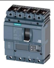
CIRCUIT BREAKER 3VA2 IEC FRAME 100 BREAKING CAPACITY CLASS H ICU=85KA @ 415 V 4POLE, LINE PROTECTION ETU860, LSIG, IN=100A OVERLOAD PROTECTION IR=40A ...100A SHORT CIRCUIT PROTECTION ISD=0,6..10X IN, II=1,5..12X IN NEUTRAL PROTECTION ADJUSTABLE (OFF, UPTO 100%) GROUNDFAULT, SWITCHABLE IG=0,2... 1 X IN, TG=0,050,8MS BUSBAR CONNECTION
