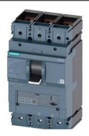
CIRCUIT BREAKER 3VA2 IEC FRAME 400 BREAKING CAPACITY CLASS H ICU=85KA @ 415 V 3-POLE, LINE PROTECTION ETU320, LI, IN=250A OVERLOAD PROTECTION IR=100A ...250A SHORT CIRCUIT PROTECTION II=12 X IN BUSBAR CONNECTION
