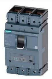
CIRCUIT BREAKER 3VA2 IEC FRAME 630 BREAKING CAPACITY CLASS M ICU=55KA @ 415 V 3-POLE, LINE PROTECTION ETU330, LIG, IN=400A OVERLOAD PROTECTION IR=160A ...400A SHORT CIRCUIT PROTECTION II=1,5...12 X IN GROUND-FAULT-PROTECTION IG=0,2... 1 X IN, TG=0,1/0,3MS BUSBAR CONNECTION
