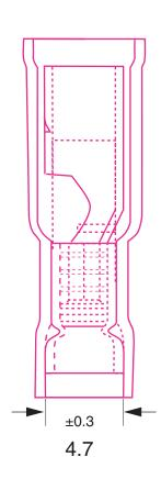
Max Electric Current: 16-14 AWG / 15 Amp Max Electric Rating: 75° C / 300 V max
