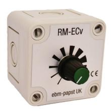
The RM-ECv controller is for use with the full range of ebm-papst EC fans. Powered by the 10V DC output from the motor, it provides infinitely variable, manual speed control between 0% and 100%.
