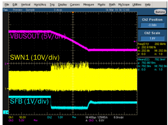
Figure 17. 12 V to 5 V Transition with No Load
