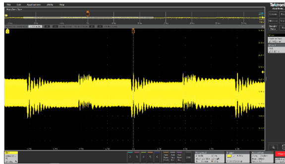
Figure 25. Transient Load on 9 V BUS
