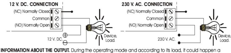
fluctuation or an incorrect working of the output. In such case, you have to install an anti-spark circuit between both contacts of the used relay, as it is indicated on the schedule.
