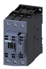
CONTACTOR,AC3:18.5KW/400V, 1NO+1NC, 230V AC 50/60HZ, 3-POLE, SIZE S2, SPRING-TYPE TERMINAL UPRIGHT MOUNTING POSITION
