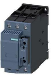
CONTACTOR, AC-6B, 75KVAR/400V, 2NC, 24V AC, 50/60HZ, 3-POLE, SIZE S2 SCREW TERMINAL
