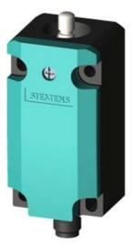
SIRIUS POSITION SWITCH, PLASTIC ENCLOSURE ACC. TO EN50041, 40MM 1NO/1NC SLOW-ACTION CONTACTS W. M12 CONNECTOR,4-POLE PIN ASSIGNMENT: PIN1=21, PIN2=22, PIN3=13,PIN4=14, MAX.250V AND 4A, TEFLON PLUNGER
