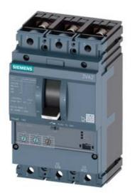
CIRCUIT BREAKER 3VA2 IEC FRAME 160 BREAKING CAPACITY CLASS C ICU=110KA @ 415 V 3POLE, LINE PROTECTION ETU320, LI, IN=100A OVERLOAD PROTECTION IR=40A ...100A SHORT CIRCUIT PROTECTION II=12 X IN BUSBAR CONNECTION
