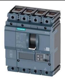
CIRCUIT BREAKER 3VA2 IEC FRAME 160 BREAKING CAPACITY CLASS M ICU=55KA @ 415 V 4POLE, LINE PROTECTION ETU560, LSIG, IN=160A OVERLOAD PROTECTION IR=64A ...160A SHORT CIRCUIT PROTECTION ISD=0,6..10X IN, II=1,5..10X IN NEUTRAL PROTECTION ADJUSTABLE (OFF, UPTO 100%) GROUNDFAULT, SWITCHABLE IG=0,2... 1 X IN, TG=0,050,8MS CABLE CONNECTION
