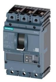
CIRCUIT BREAKER 3VA2 IEC FRAME 250 BREAKING CAPACITY CLASS M ICU=55KA @ 415 V 3POLE, LINE PROTECTION ETU860, LSIG, IN=160A OVERLOAD PROTECTION IR=64A ...160A SHORT CIRCUIT PROTECTION ISD=0,6..10X IN, II=1,5..12X IN NEUTRAL PROTECTION OPTIONAL WITH EXT. CT,UPTO 160% GROUNDFAULT, SWITCHABLE IG=0,2... 1 X IN, TG=0,050,8MS BUSBAR CONNECTION
