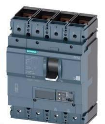
CIRCUIT BREAKER 3VA2 IEC FRAME 400 BREAKING CAPACITY CLASS M ICU=55KA @ 415 V 4-POLE, LINE PROTECTION ETU860, LSIG, IN=400A OVERLOAD PROTECTION IR=160A ...400A SHORT CIRCUIT PROTECTION ISD=0,6..10X IN, II=1,5..10X IN NEUTRAL PROTECTION ADJUSTABLE (OFF, UPTO 100%) GROUND-FAULT, SWITCHABLE IG=0,2... 1 X IN, TG=0,05-0,8MS BUSBAR CONNECTION
