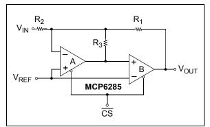
FIGURE 4-17: Capacitorless Second-Order Low-Pass Filter with Chip Select.
