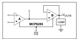
FIGURE 4-10: Isolating the Load with a Buffer.
