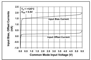
**FIGURE 2-12:** Input Bias, Offset Currents vs. Common Mode Input Voltage at  $T_A = +125^{\circ}C$ .
