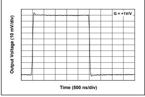
*FIGURE 2-26:* Small-Signal, Non-inverting Pulse Response.
