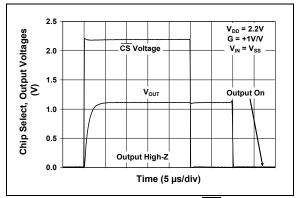
**FIGURE 2-27:** Chip Select  $(\overline{CS})$  to Amplifier Output Response Time at  $V_{DD} = 2.2V$ (MCP6283 and MCP6285 only).
