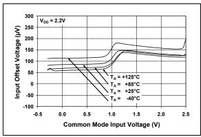
**FIGURE 2-3:** Input Offset Voltage vs. Common Mode Input Voltage at  $V_{DD} = 2.2V$ .
