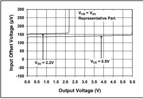
FIGURE 2-7: Input Offset Voltage vs. Output Voltage.
