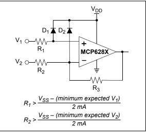
FIGURE 4-2: Protecting the Analog Inputs.
