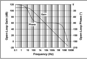
FIGURE 2-14: Open-Loop Gain, Phase vs. Frequency.
