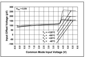
**FIGURE 2-6:** Input Offset Voltage vs. Common Mode Input Voltage at  $V_{DD}$  = 5.5V.
