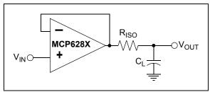
*FIGURE 4-3:* Output Resistor, R<sub>ISO</sub> stabilizes large capacitive loads.
