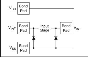
FIGURE 4-1: Simplified Analog Input ESD Structures.
