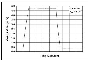
*FIGURE 2-25:* Large-Signal, Non-inverting Pulse Response.
