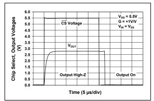
**FIGURE 2-30:** Chip Select ( $\overline{CS}$ ) to Amplifier Output Response Time at V<sub>DD</sub> = 5.5V (MCP6283 and MCP6285 only).
