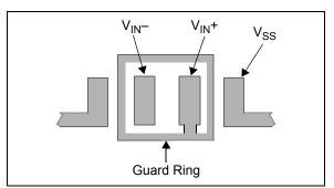
**FIGURE 4-7:** Example Guard Ring Layout for Inverting Gain.
