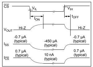
**FIGURE 1-1:** Timing Diagram for the Chip Select (CS) pin on the MCP6283 and MCP6285.
