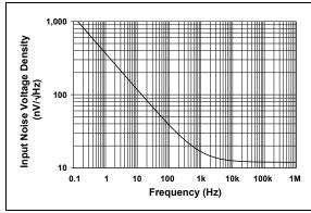
FIGURE 2-19: Input Noise Voltage Density vs. Frequency.
