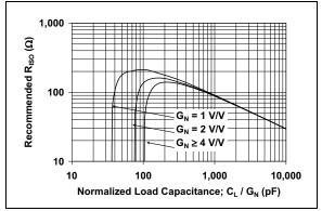
**FIGURE 4-4:** Recommended R<sub>ISO</sub> Values for Capacitive Loads.
