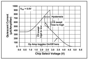
FIGURE 2-24:Quiescent Current vs.Chip Select (CS)Voltage at  $V_{DD}$  = 5.5V(MCP6283 and MCP6285 only).
