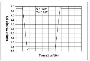
**FIGURE 2-28:** Large-Signal, Inverting Pulse Response.
