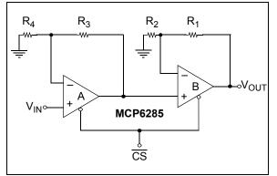
FIGURE 4-11: Cascaded Gain Circuit Configuration.
