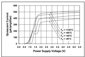
**FIGURE 2-13:** Quiescent Current vs. Power Supply Voltage.
