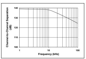
**FIGURE 2-23:** Channel-to-Channel Separation vs. Frequency (MCP6282 and MCP6284 only).
