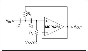
FIGURE 4-8: Sallen-Key High-Pass Filter.
