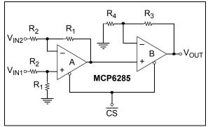
FIGURE 4-12: Difference Amplifier Circuit.
