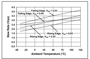
FIGURE 2-18:Slew Rate vs. AmbientTemperature.
