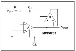
**FIGURE 4-14:** Integrator Circuit with Active Compensation.
