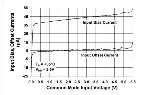
**FIGURE 2-9:** Input Bias, Offset Currents vs. Common Mode Input Voltage at  $T_A = +85^{\circ}C$ .
