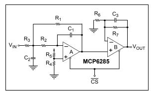
**FIGURE 4-15:** Second-Order Multiple Feedback Low-Pass Filter with an Extra Pole-Zero Pair.
