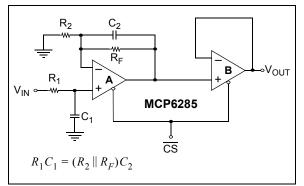
FIGURE 4-13: Buffered Non-inverting Integrator with Chip Select.
