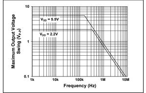
FIGURE 2-15: Maximum Output Voltage Swing vs. Frequency.
