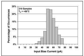
**FIGURE 2-2:** Input Bias Current at  $T_A = +85$  °C.
