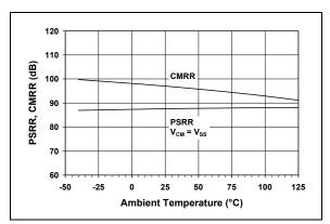
*FIGURE 2-11:* CMRR, PSRR vs. Ambient Temperature.
