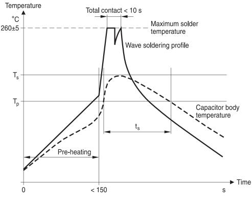
$T_{s}: Capacitor body maximum temperature at wave soldering \\T_{p}: Capacitor body maximum temperature at pre-heating \\ KMK1745-A-E$
