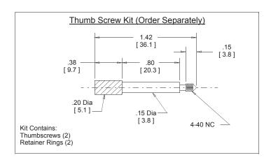
$Note: The \ 3M^{\text{TM}} \ 3341-7 \ Thumb \ Screw \ contains \ lead \ in \ the \ base \ material, therefore \ RIAE5 \&C3 \ apply \ when \ using \ this \ hardware.$
