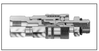
The FD90 Series diagnostic coupling is designed to connect and disconnect pressure gauges to hydraulic systems, eliminating the need for permanent gauges. The maximum operating pressure is 7,000 psi.
