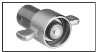
As the number of applications for couplings grew, so did the demand for reduced spillage. Aeroquip responded with the patented tubular valve design which became standard in critical industrial and aerospace applications. Typically, fluid loss is measured in fractions of cc's per disconnection.
