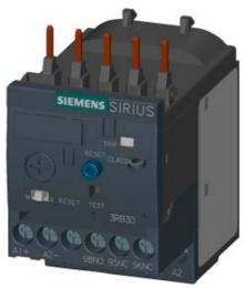
OVERLOAD RELAY 4...16 A FOR MOTOR PROTECTION SIZE S00, CLASS 10 CONTACTOR ASS. MAIN CIRCUIT: SCREW CONN. AUX.CIRCUIT: SCREW CONN. MANUAL-AUTOM.-RESET
