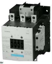
CONTACTOR, 55KW/400V/AC-3, AC(40...60HZ)/DC OPERATION UC 575...600V AUXIL. CONTACTS 2NO+2NC 3-POLE, SIZE S6 BAR CONNECTIONS CONVENTIONAL OPERATING MECHAN. SCREW TERMINAL
