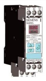
DIGITAL MONITORING RELAY CURRENT MONITORING, 22.5MM FROM 2 TO 500MA AC/DC OVERSHOOT AND UNDERSHOOT SUPPLY VOLTAGE: AC/DC 24V DC AND AC 50 TO 60 HZ NO GALVANIC ISOLATION FROM MEASURING CIRCUIT STARTUP AND INTERF. PEAK DELAY 0.1 TO 20S HYSTERESIS 0.1 TO 250MA 1 CO CONTACT W. OR W/O ERROR LOG SCREW TERMINAL REPLACEMENT PRODUCT FOR 3UG3521-1AC..
