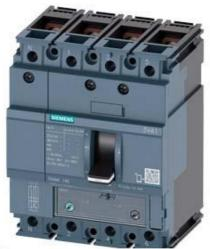
CIRCUIT BREAKER 3VA1 IEC FRAME 160 BREAKING CAPACITY CLASS N ICU=25KA @ 415 V 4-POLE, LINE PROTECTION TM240, ATAM, IN=80A OVERLOAD PROTECTION IR=56A ...80A SHORT CIRCUIT PROTECTION II=5...10 X IN NEUTRAL UNPROTECTED BUSBAR CONNECTION
