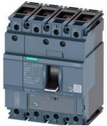
CIRCUIT BREAKER 3VA1 IEC FRAME 160 BREAKING CAPACITY CLASS N ICU=25KA @ 415 V 4-POLE, LINE PROTECTION TM220, ATFM, IN=16A OVERLOAD PROTECTION IR=11,2A ...16A SHORT CIRCUIT PROTECTION II=10 X IN NEUTRAL UNPROTECTED BUSBAR CONNECTION
