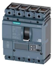
CIRCUIT BREAKER 3VA2 IEC FRAME 160 BREAKING CAPACITY CLASS M ICU=55KA @ 415 V 4POLE, LINE PROTECTION ETU850, LSI, IN=25A OVERLOAD PROTECTION IR=10A ...25A SHORT CIRCUIT PROTECTION ISD=0,6..10X IN, II=1,5..12X IN NEUTRAL PROTECTION ADJUSTABLE (OFF, UPTO 160%) CABLE CONNECTION
