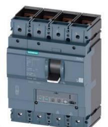
CIRCUIT BREAKER 3VA2 IEC FRAME 400 BREAKING CAPACITY CLASS H ICU=85KA @ 415 V 4-POLE, LINE PROTECTION ETU330, LIG, IN=400A OVERLOAD PROTECTION IR=160A ...400A SHORT CIRCUIT PROTECTION II=1,5...10 X IN NEUTRAL PROTECTION ADJUSTABLE(OFF,50%,100%) GROUND-FAULT-PROTECTION IG=0,2... 1 X IN, TG=0,1/0,3MS BUSBAR CONNECTION
