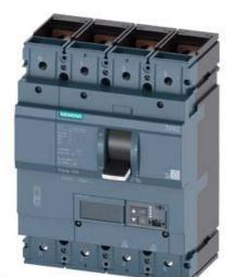
CIRCUIT BREAKER 3VA2 IEC FRAME 630 BREAKING CAPACITY CLASS M ICU=55KA @ 415 V 4-POLE, LINE PROTECTION ETU560, LSIG, IN=500A OVERLOAD PROTECTION IR=200A ...500A SHORT CIRCUIT PROTECTION ISD=0,6..10X IN, II=1,5..14X IN NEUTRAL PROTECTION ADJUSTABLE (OFF, UPTO 100%) GROUND-FAULT, SWITCHABLE IG=0,2... 1 X IN, TG=0,05-0,8MS BUSBAR CONNECTION
