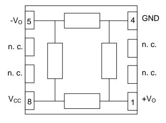
Figure 2: internal and external connections (TDFN, Chip)
