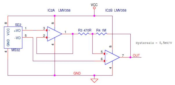
Figure 6: Switching point detection with hysteresis
