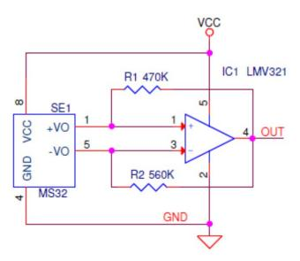
Figure 5: Switching point detection without hysteresis
