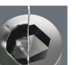
Hexagon socket screws are a problem, because the contact surfaces that transfer the force of the tool to the screw are very narrow. The consequence: the head of the screw can be damaged, usually rounding out the recess. Hex-Plus tools have larger contact surfaces to prevent this, driving from the flats of the recess, rather than the corners. Good to know: Hex-Plus tools fit into every standard hexagon socket screw!
