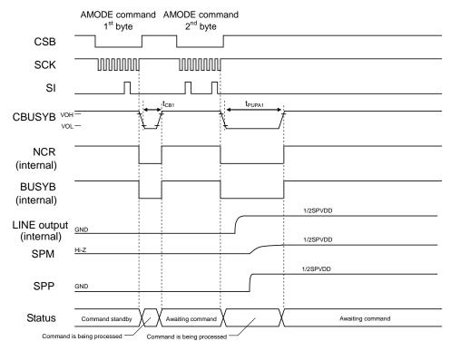
• Speaker amplifier power-up timing (DAMP bit = "1", AEN1 bit = "0", AEN0 bit = "0"  $\rightarrow$  "1")
