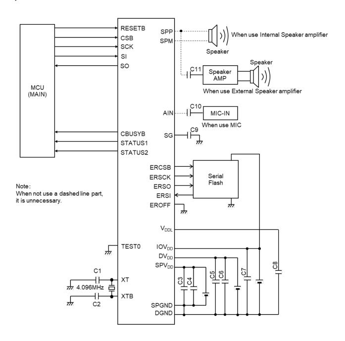
Please add necessary bypass capacitor to a power supply pin of the serial flash memory separately.
