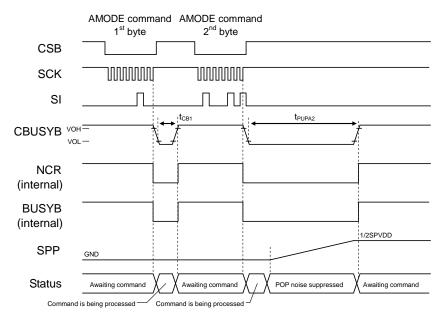
• Line amplifier power-up timing (DAMP bit = "0", POP bit = "0", AEN1 bit = "0"  $\rightarrow$  "1", AEN0 bit = "0")
