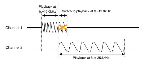
Figure 1) Case where a phrase is played at a sampling frequency belonging to a different sampling frequency group during playback on channels 1 and 2
