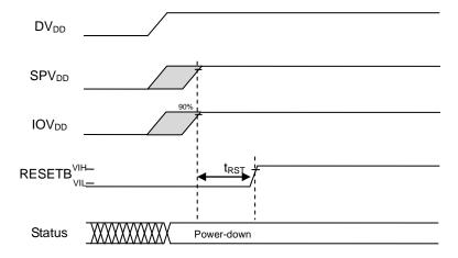
After the power is turned on, the device enters the power-down state.
