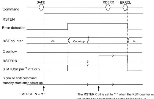
The RSTERR bit is set to "1" when the RST-counter overflows. No shifting to command wait state after power-up
