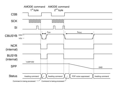
• Line amplifier power-down timing (DAMP bit = "0", POP bit = "0", AEN1 bit = "1" → "0", AEN0 bit = "0")
