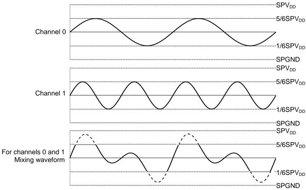
If the result of mixing channels 0 and 1 exceeds from the  $1/6SPV_{DD}$  to 5/6SPVDD level (as indicated by the broken line), the sound quality may be reduced by clamping. Waveforms when AVOL is set to 0.0dB.
