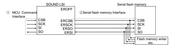
① Rewrite using the clock synchronous serial interface of the MCU command interface By using the CSB, SCK, SI and SO pins, which are clock synchronous serial interfaces of the MCU command interface the serial flash memory can be rewritten. When the PUP command and FDIRECT command are entered with the EROFF pin set to "L", direct access to the serial flash memory is enabled from the CSB, SCK, SI and SO pins.
