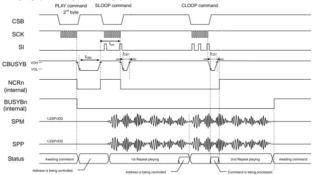
The SLOOP command is valid only during playback. After the PLAY command is input, input the SLOOP command within the specified period ( $t_{cm}$ ) after the NCR of the corresponding channel becomes "H" level. This enables the SLOOP command and repeats playback. While the repeat playback mode is set, the NCR signal is "L" level.
