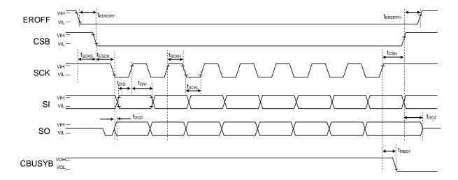
◆ Clock Synchronous Serial Interface Timing (SCK Initial Value = "L" Level)
