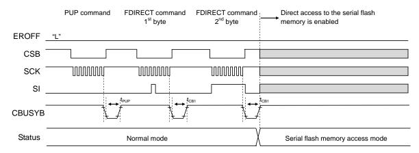
For the PUP command, refer to the "PUP command" in the "Command" section. For the FDIRECT command, refer to the "FDIRECT command" in the "Command" section.
