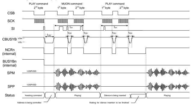
After the PLAY command is input, the CBUSYB signal and NCR signal change to "H" level when the address management of phrase 1 is completed and start playing back. Input the MUON command after the CBUSYB signal changed to "H" level. After the MUON command is received, the LSI is in a state waiting for the end of playback of phrase 1 and the NCR signal remains "L" level until the end of playback.
