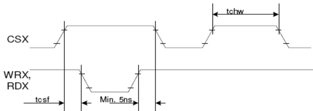
*Note: Logic high and low levels are specified as 30% and 70% of IOVCC for Input signals.*
