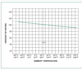
Note: 1. Rerating depicted in this curve is in addition to the standard derating of 25% for continuous operation.
