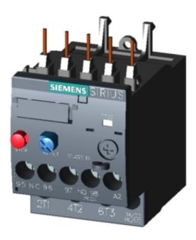
OVERLOAD RELAY 1.4...2.0 A FOR MOTOR PROTECTION SZ S00, CLASS 10, F. MOUNTING ONTO CONTACTOR MAIN CIRCUIT: SCREW TERMINAL AUX. CIRCUIT: SCREW TERMINAL MANUAL-AUTOMATIC-RESET
