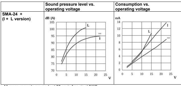
All measurements are made at 30 cm in free air at 21°C.
