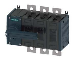
SWITCH-DISCONNECTOR 250A, FRAME SIZE 3, 3-POLE FRONT OPERATING LEFT COMPLETE ASSEMBLY WITH DIRECT HANDLE GREY FLAT TERMINAL
