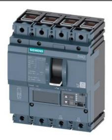
CIRCUIT BREAKER 3VA2 IEC FRAME 160 BREAKING CAPACITY CLASS M ICU=55KA @ 415 V 4POLE, LINE PROTECTION ETU860, LSIG, IN=40A OVERLOAD PROTECTION IR=16A ...40A SHORT CIRCUIT PROTECTION ISD=0,6..10X IN, II=1,5...12X IN NEUTRAL PROTECTION ADJUSTABLE (OFF, UPTO 160%) GROUNDFAULT, SWITCHABLE IG=0,2... 1 X IN, TG=0,050,8MS CABLE CONNECTION
