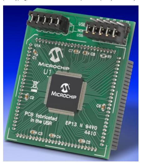
The capabilities of PIC32MX1/2 XLP family of devices can be demonstrated with the PIC32MX274F256 PIM using Explorer 16 development board. It enables USB and demonstrates the low power sleep and deep sleep features of the PIC32MX XLP series.
