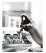
When doing screwdriving jobs on electronic components (like e.g. smartphones and tablet PCs), there should be no electrostatic discharge as this could cause malfunctions and a complete failure. Therefore, tools that are secure against electrostatic discharge are indispensable.
