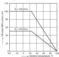
1–5.ON–state RMS current vs. ambient temperature characteristics
