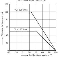
1–6.ON–state RMS current vs. ambient temperature characteristics
