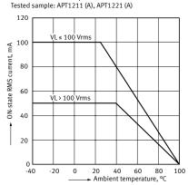
1–4.ON–state RMS current vs. ambient temperature characteristics
