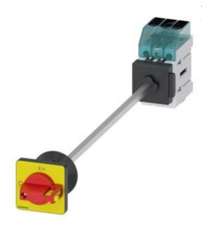
Switch disconnector 3LD3, main switch 3-polig, lu 63A operational switch at AC-23 A at 400 V 22,0 kW floor mounting Base mounting with door coupling center-hole 22,5 mm knob-operated mechanism red/yellow 48 x 48 mm
