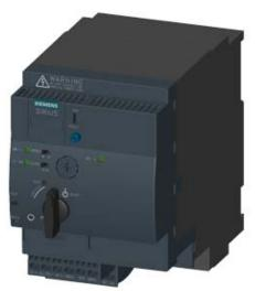
SIRIUS, COMPACT STARTER, REVERSING STARTER 690 V, 110 ... 240 V AC/DC, 50 ... 60 HZ, 0.32 ... 1.25 A, IP20, MAIN CIRCUIT CONNECTION: PLUG-IN, W/O TERMINALS, AUXILIARY CIRCUIT CONNECTION: SPRING-LOADED TERMINAL
