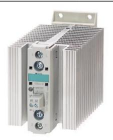
SEMI-COND. CONTACTOR 3RF2,1-PH. AC 51 40 A 40 DEGREES C 24-230 V / 24 V DC SCREW TERMINAL
