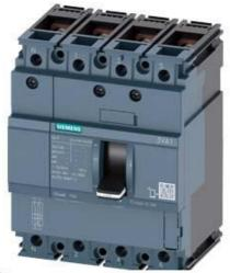
CIRCUIT BREAKER 3VA1 IEC FRAME 100 BREAKING CAPACITY CLASS S ICU=36KA @ 415 V 4-POLE, LINE PROTECTION TM210, FTFM, IN=80A OVERLOAD PROTECTION IR=80A FIXED SHORT CIRCUIT PROTECTION II=10 X IN NEUTRAL UNPROTECTED BUSBAR CONNECTION
