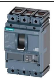
CIRCUIT BREAKER 3VA2 IEC FRAME 100 BREAKING CAPACITY CLASS C ICU=110KA @ 415 V 3POLE, LINE PROTECTION ETU560, LSIG, IN=100A OVERLOAD PROTECTION IR=40A ...100A SHORT CIRCUIT PROTECTION ISD=0,6..10X IN, II=1,5...12X IN NEUTRAL PROTECTION OPTIONAL WITH EXT. CT,UPTO 160% GROUNDFAULT, SWITCHABLE IG=0,2... 1 X IN, TG=0,050,8MS CABLE CONNECTION
