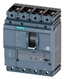
CIRCUIT BREAKER 3VA2 IEC FRAME 100 BREAKING CAPACITY CLASS M ICU=55KA @ 415 V 4POLE, LINE PROTECTION ETU350, LSI, IN=40A OVERLOAD PROTECTION IR=16A ...40A SHORT CIRCUIT PROTECTION ISD=1,5... 10 X IR, II=12 X IN NEUTRAL PROTECTION ADJUSTABLE(OFF,100%) BUSBAR CONNECTION
